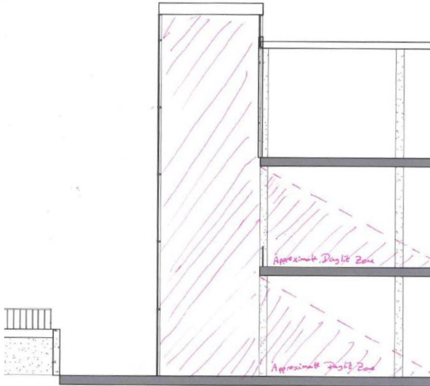
Figure 1 – Sketch of Approximate Daylight Zone (in Elevation)
